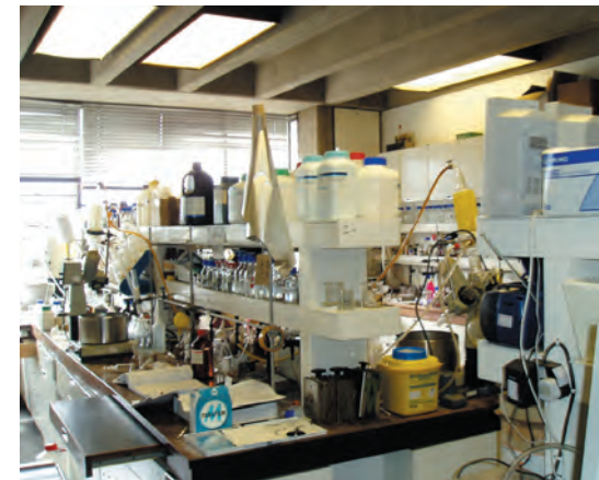
Some chemistry laboratories retain the original fittings of the 1960s, but the laboratories are being refitted using more modern equipment. Note ceiling of exposed, unpainted precast concrete T-beam and original light fittings.
