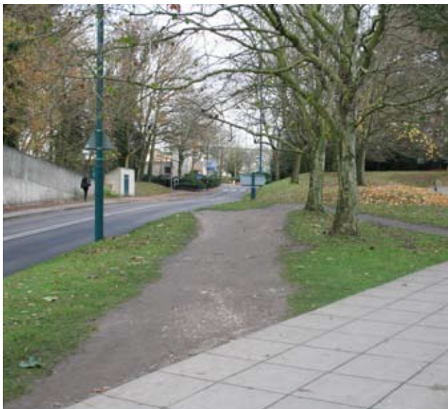
Below: Erosion caused by the trampling on a desire line
