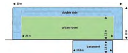
Diagram showing the overall dimensions of SCVA [7] and the urban room. About 45% of the volume of building is taken up with service areas in the double skin and basement.
