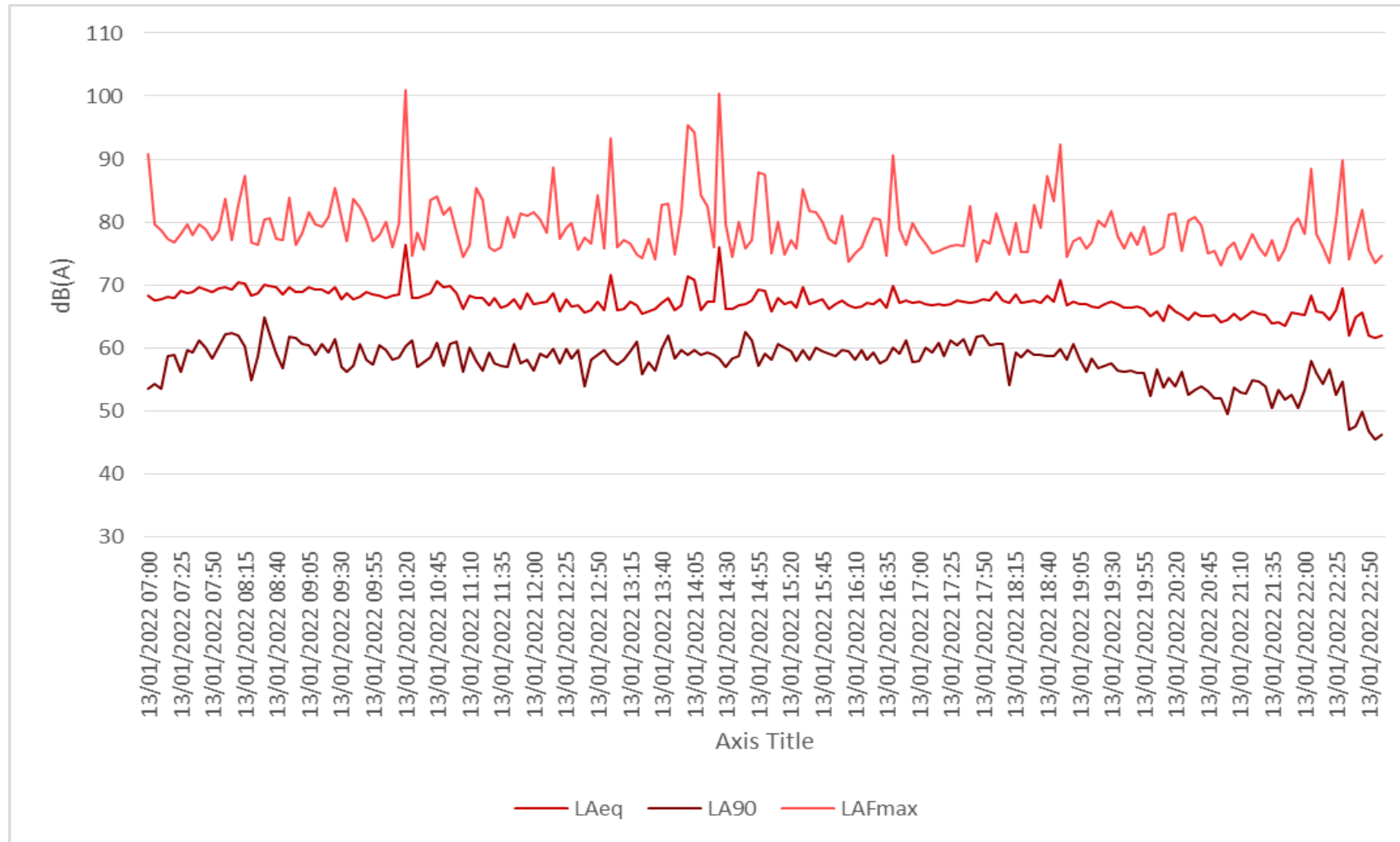
Graph 14: Graphical representation of the 16 hour noise monitoring period (07:00-23:00) on 13 th January 2022 (New Botolph Street)
