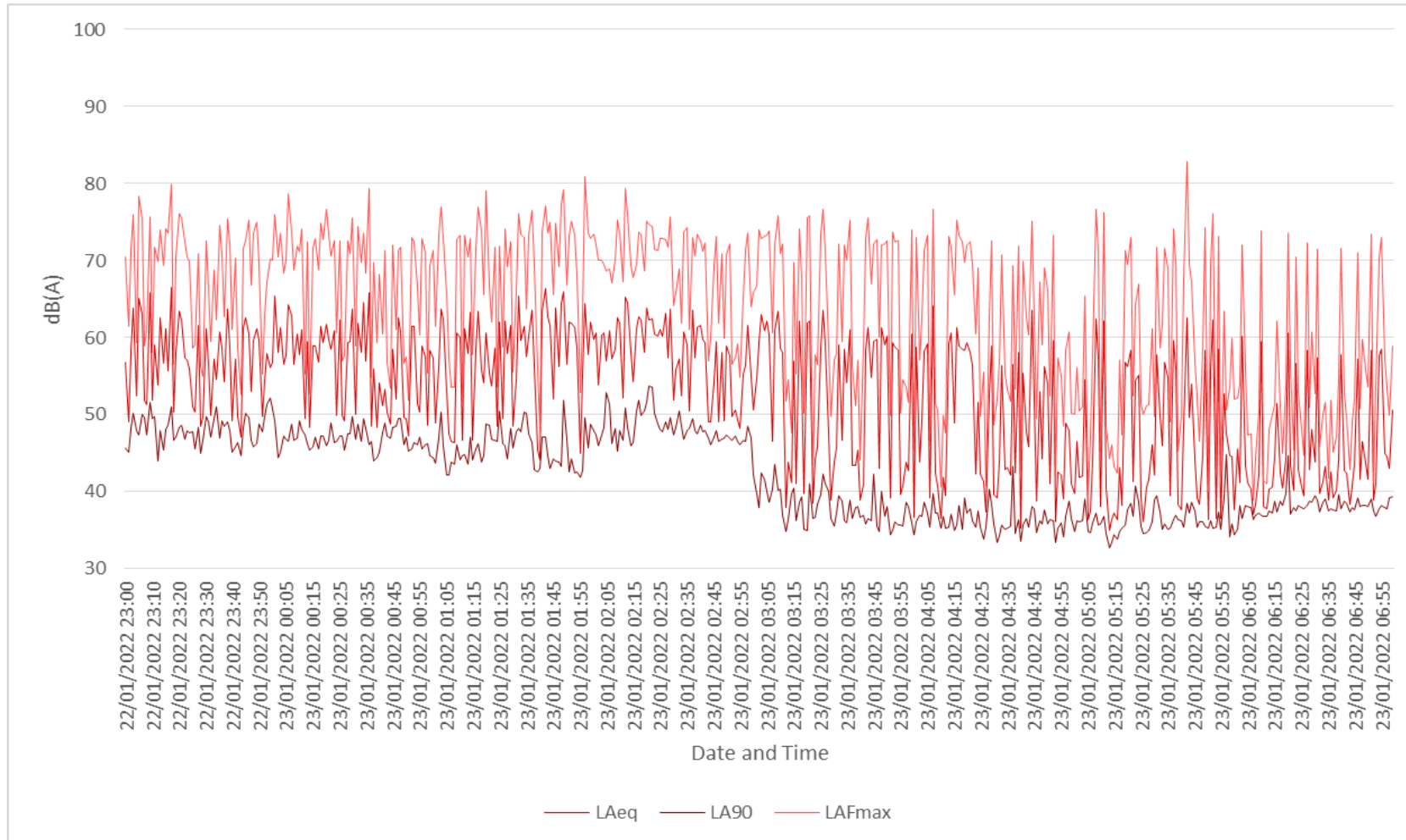
Graph 32: Graphical representation of the night monitoring period (8 hour) on the 22 nd / 23 rd January 2022 (Edward Street)
