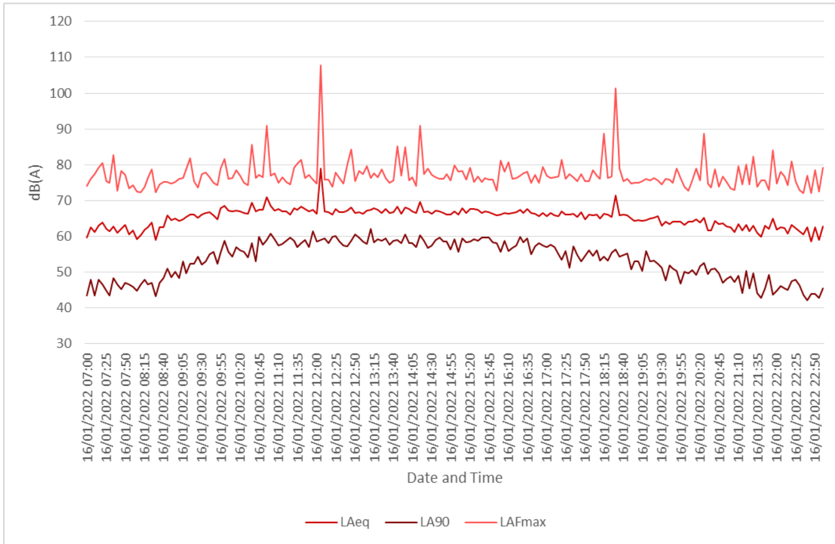
Graph 16: Graphical representation of the 16hour noise monitoring period (07:00-23:00) on 16 th January 2022 (New Botolph Street)
