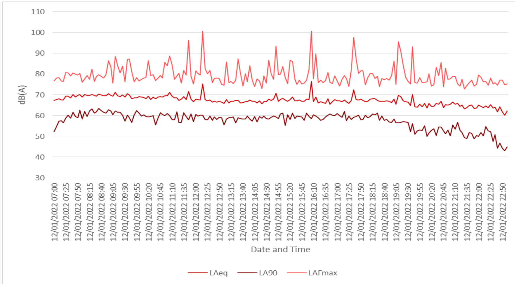
Graph 13: Graphical representation of the 16 hour noise monitoring period (07:00-23:00) on 12 th January 2022 (New Botolph Street)
