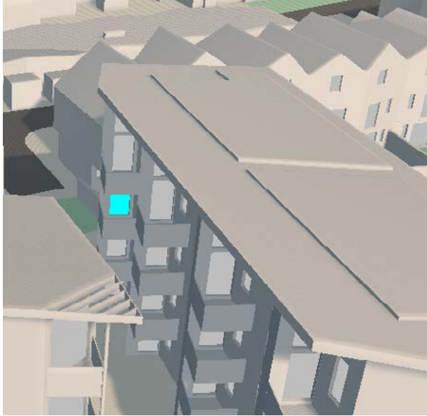
Figure 14: Window Map for W2/F02 and Waldram diagram highlighting how the existing overhanging balcony feature restricts the receipt of daylight.
