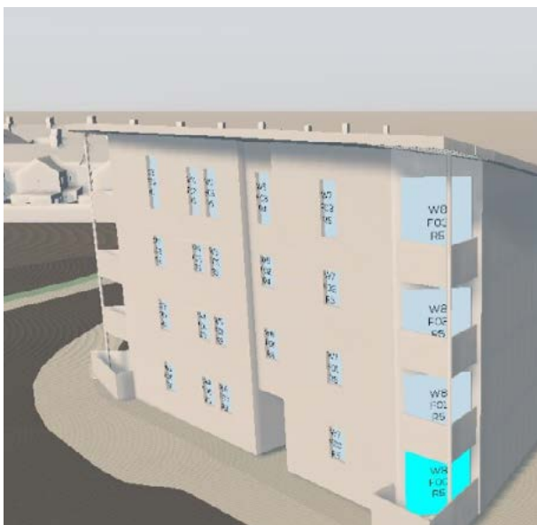
Figure 12: Window Map for W8/F00 and Waldram diagram highlighting how the existing overhanging balcony feature restricts the receipt of daylight.
