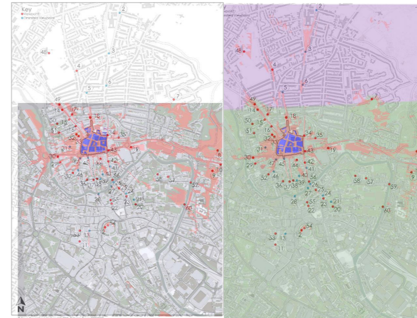
Figure 1: Comparison (as an overlay with the original 62 views assessed with the Appeal Scheme) of the ZVI produced by the massing as it stood in October 2021 (left) and February 2022 (right).
