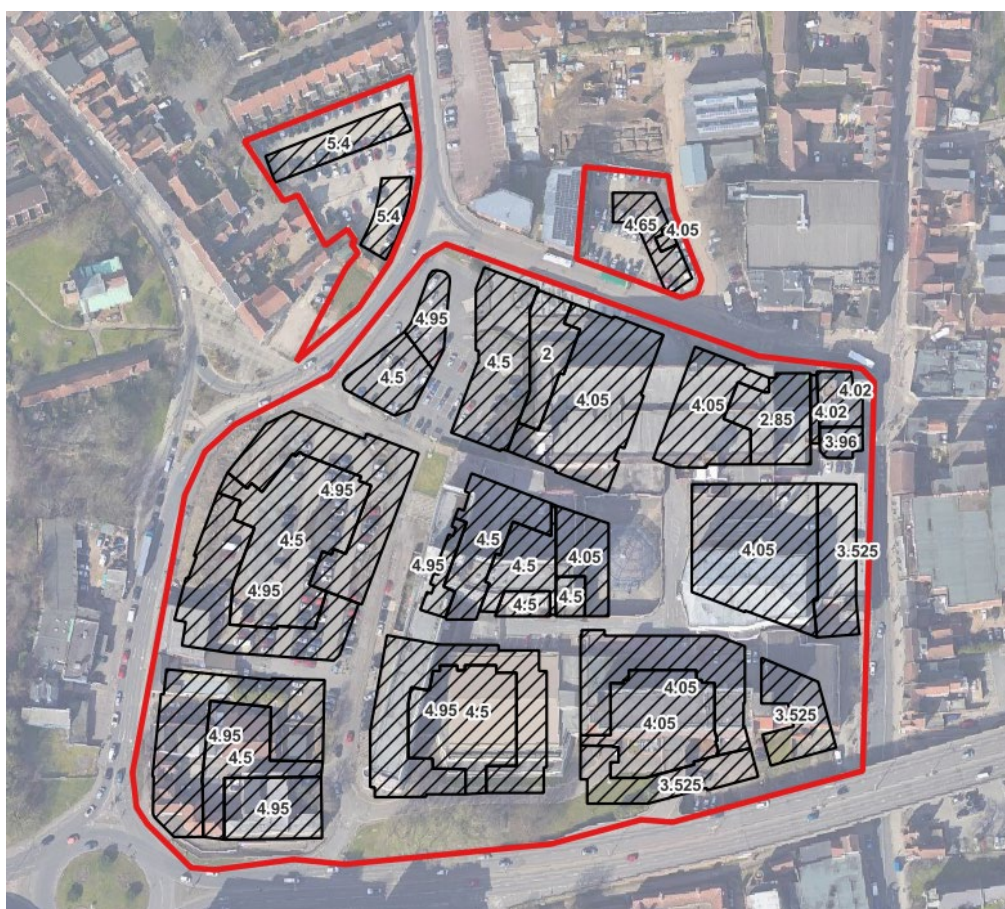
Figure 5: Illustrative finished floor levels for each block represented in Anglia Square model (m AOD)
