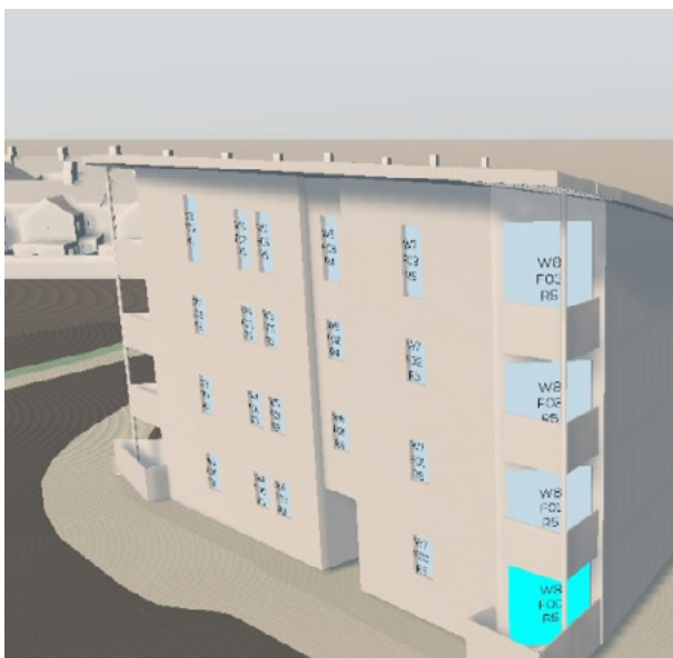
Figure 09: Window Map for W8/F00 and Waldram diagram highlighting how the existing overhanging balcony feature restricts the receipt of daylight.
