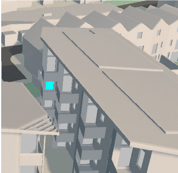
Figure 11: Window Map for W2/F02 and Waldram diagram highlighting how the existing overhanging balcony feature restricts the receipt of daylight.
