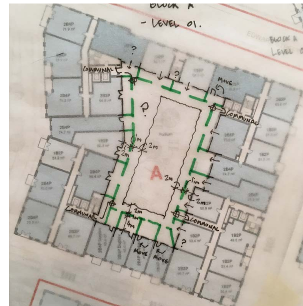
Setting a private demised area.
