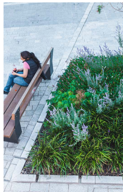
Planting bed with infiltration kerb
