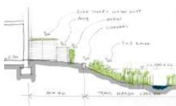
Private back garden with 1.8m high bike store, step down AHU housing and 1.4m post and rail fence
