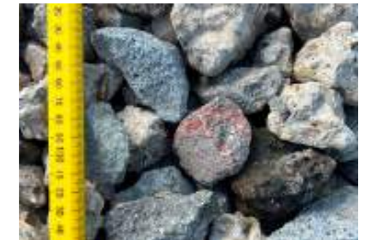
Gabions could be made with material sourced during site clearance
