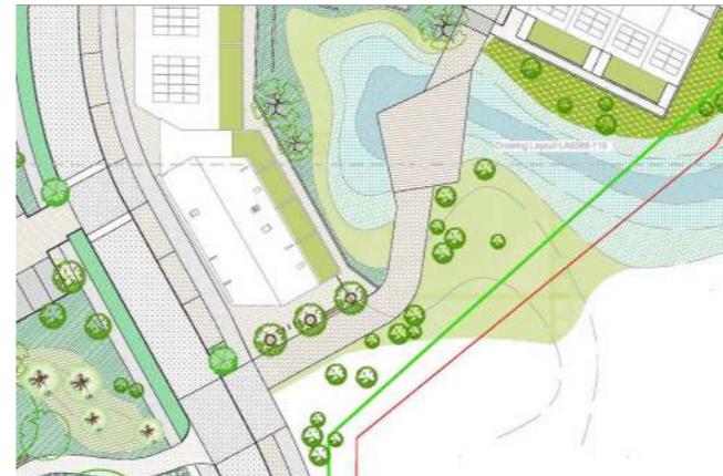
2. Decking areas over the bio swales provide additional public space along the cycleway
