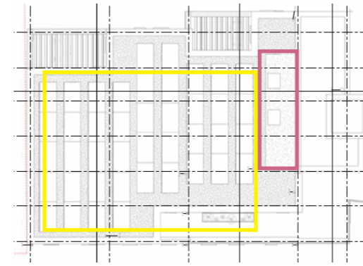
Typical placement of AHUs and solar panels on roof
