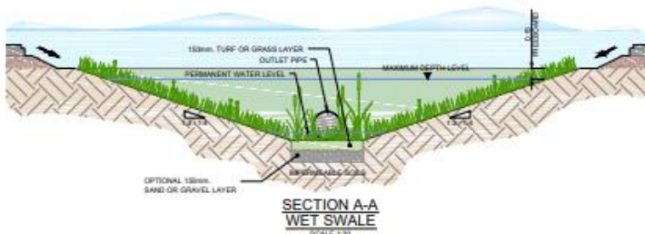
H2-A - Typical swale details
