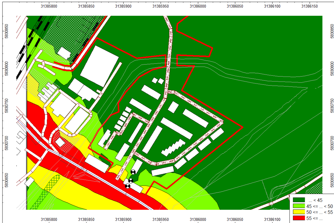
Figure 28 – May Gurney: AVO Guide Level 2 assessment recommended (night-time)
