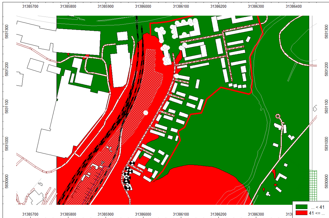
Figure 30 – Exceedances of ADO L_{night} criterion due to conveyor at Trowse Depot
