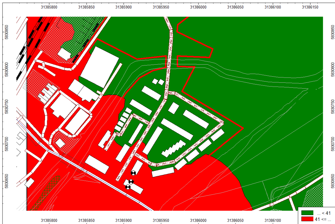
Figure 31 – Exceedances of ADO L_{night} criterion in May Gurney due to traffic noise
