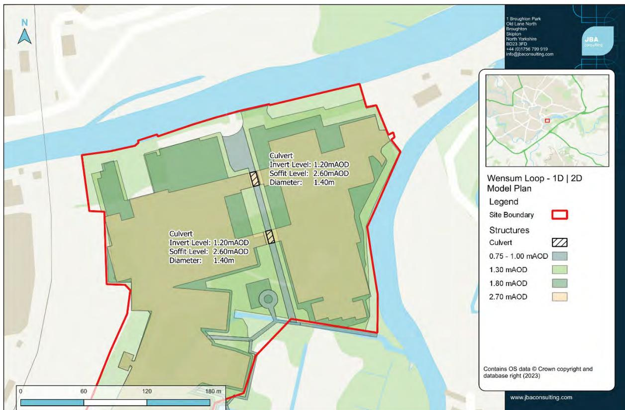
Figure 7-4: Wensum Loop - Flow route / culvert arrangement
