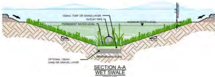
H2-A - Typical swale details
