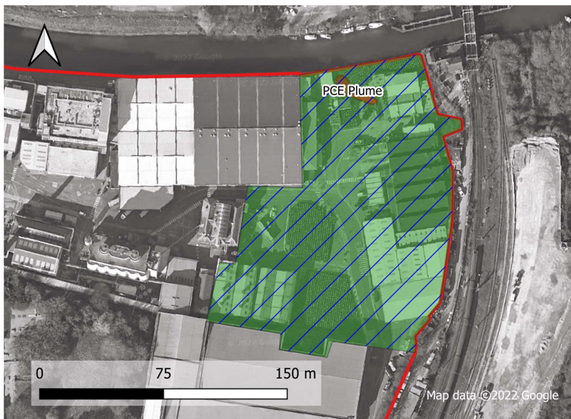
Figure 12.13: PCE Plume and Remediation Area
