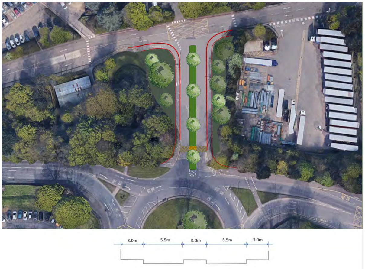
Figure 4.7 – Carrow Works parallel carriageway initial design concept.
