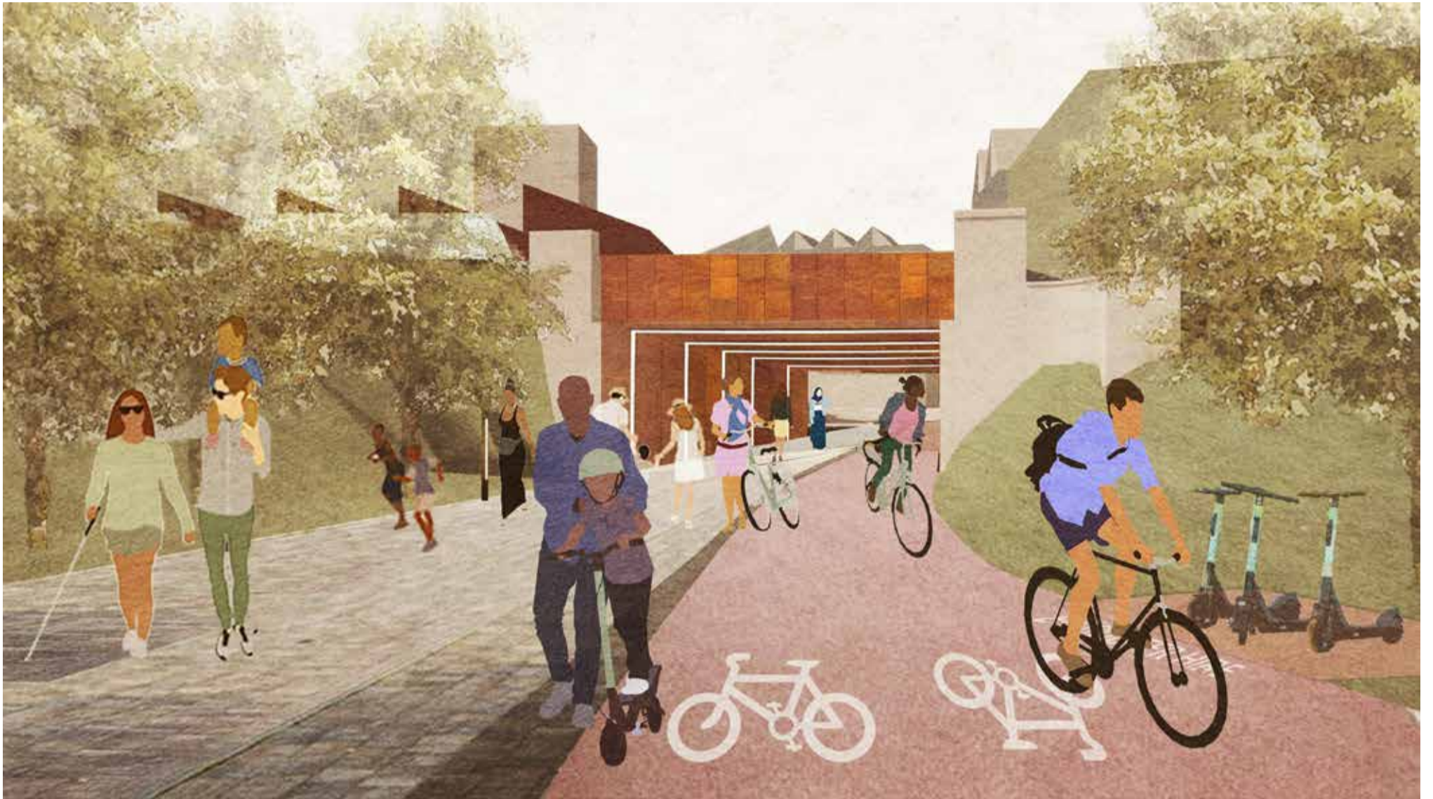
Existing tunnel location widened to 6m and excavated to 2.7m deep. Option using corten steel and lighting to create a light and inviting space to connect the masterplan.
