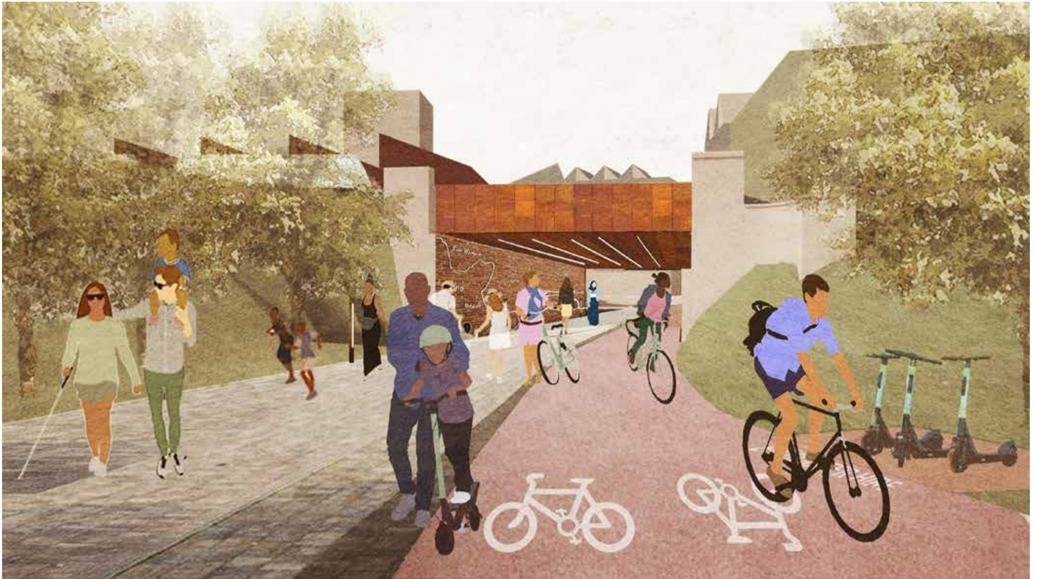
Existing tunnel location widened to 6m and excavated to 2.7m deep. Option using brickwork and lighting, potential mural or artwork installation to inner wall, which could link to local history.
