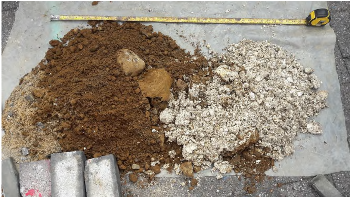
Plate 5: Very shallow natural weathered structureless chalk below 0.53m at WS15, Area 11.
