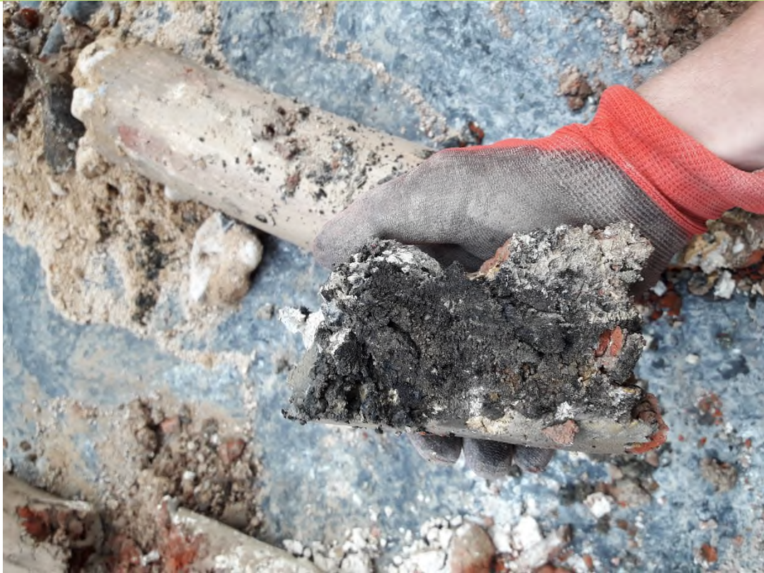
Plate 9: Black patch with a strong hydrocarbon odour between 1.40-1.90m at WS19, Area 15.
