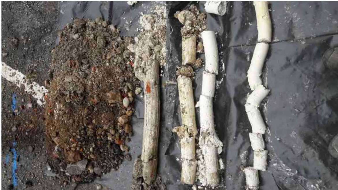
Plate 3: Made ground over natural chalk at WS4, Area 14.
