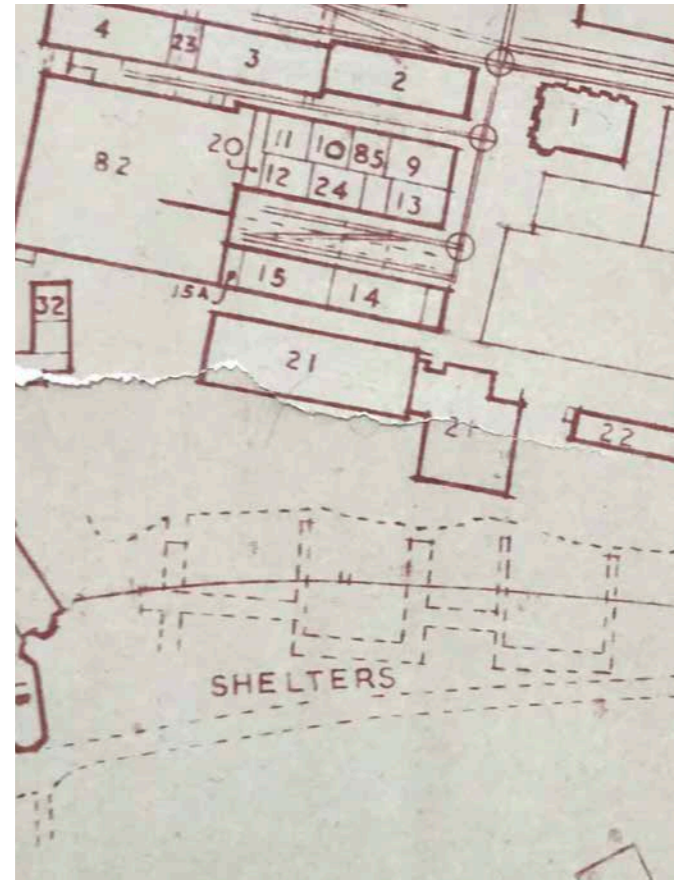
Figure 4.17 Detail of undated Block Plan showing the original configuration of the Air Raid Shelters Norfolk Record Office
