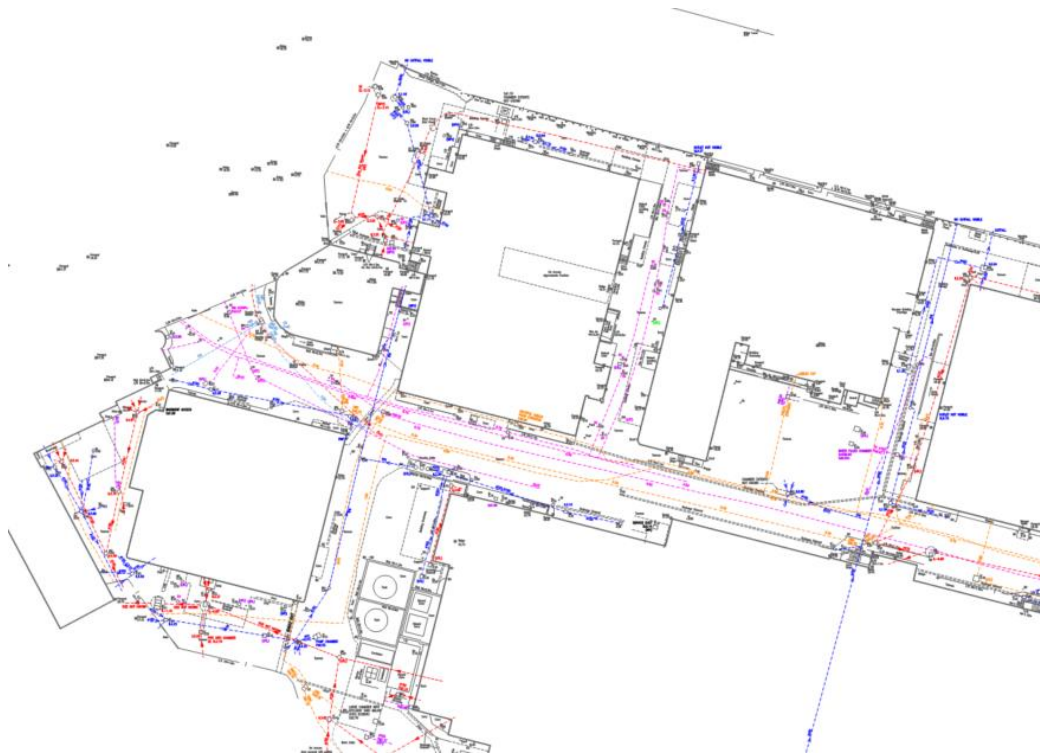
Figure 3-3: GPR Survey for Existing Surface Water Drainage (Blue) for Northern Area of Site (1 of 3)
