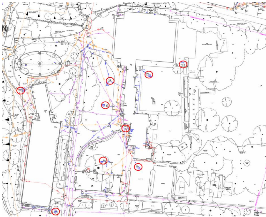
Figure 3-6: GPR Survey for Existing Surface Water Drainage (Blue) for Soakaways in Carrow Abbey
