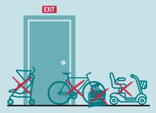
Avoid storing or charging devices with lithium batteries (mobility scooters, e-bikes, and e-scooters) indoors. If indoor charging is necessary, choose a room with a closable door. Avoid locations that may obstruct your exit, such as hallways or communal areas.
